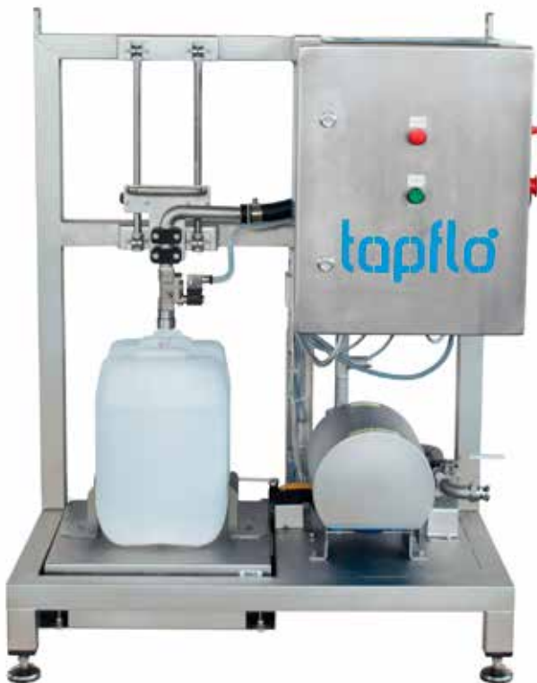
Filling Machine, bottom arrangement
